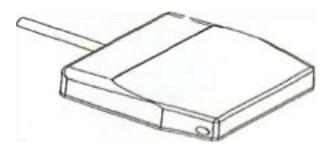
Foot Switch fully depressed the ultrasonic tip is activated and irrigating water flows.
