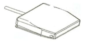
Foot Switch Released... Both ultrasonic activation and irrigating flow stop.
