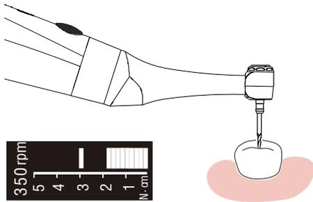
In the standby mode, the root canal preparation device is started by pressing the main switch
